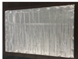
Heat insulation on skirt
