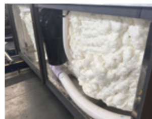
Foam insulation on tub body
